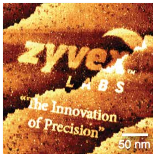
4. The final atomic-resolution pattern of exposed Si dangling bonds.
