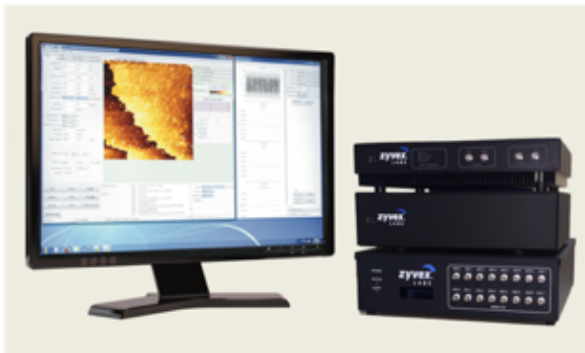
Figure 2.1: ZyVector System. Top: Analog High Voltage Box. Middle: Power Supply. Bottom: DSP.
