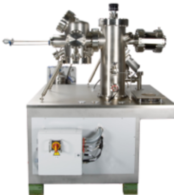
Figure 2.2 One configuration of the Omicron VT STM. (reprinted here with the permission of ScientaOmicron)
