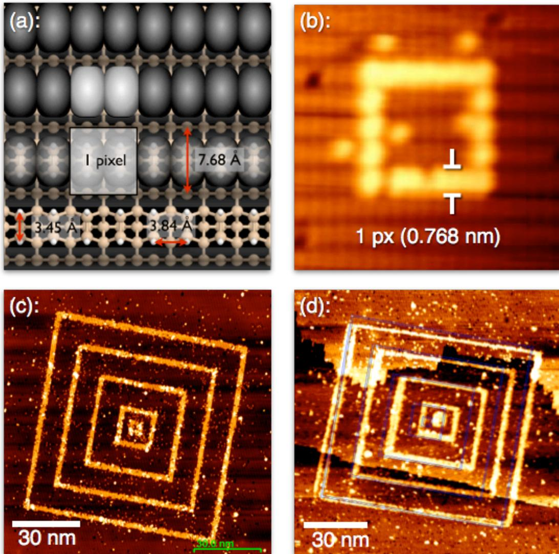
Figure 1: (a): We have defined a lithography pixel as a pair of Si dimers on a single dimer, giving a square pixel 7.68 Å wide. (b): STM lithography of a box, with a linewidth of 1 px. (c,d): A test pattern comprising 5 pairs of 1-px rectangles, largest is 112 px (86 nmwide), drawn with and without creep correction applied, respectively.
